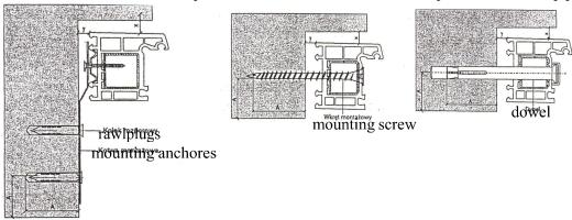
Drawing 1. A – you must apply to the producers guidelines, attachments and construction materials
